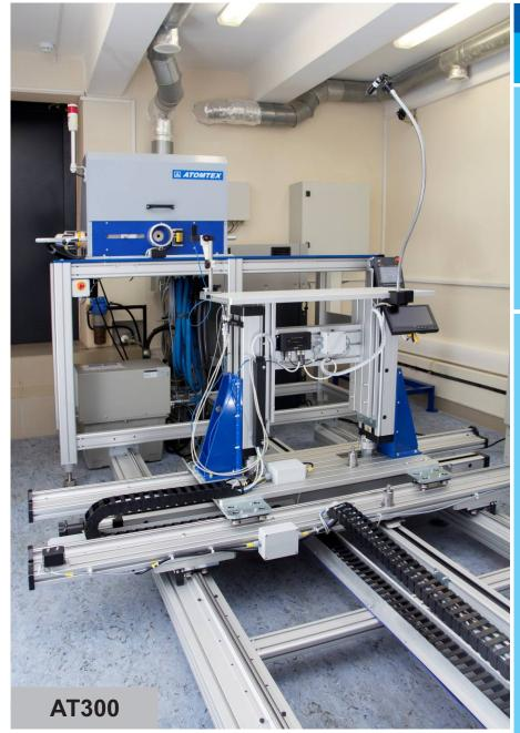
X-ray calibration system is designed to calibrate and test standards and measurement instruments in units of air kerma and air kerma rate, ambient dose equivalent and ambient dose equivalent rate, individual dose equivalent and individual dose equivalent rate, directional dose equivalent and directed dose equivalent rate of X-ray radiation.
