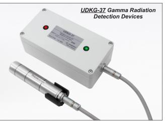
The system is based on *UDKG-37* Gamma radiation detection devices, *AT1123* X-ray and gamma radiation dosimeters and components of the AT2327 Alarm dosimeter. The *UDKG-37* detection device consists of the *BDKG-37* Gamma radiation detection unit and the *IU-37* Interface unit. Each measuring channel supports connection of an optional electronic information display.
