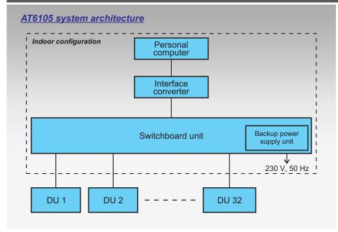
This stationary system is designed for continuous and uninterrupted dosimetric and spectrometric radiation monitoring of land, facilities, wells and other sites.
