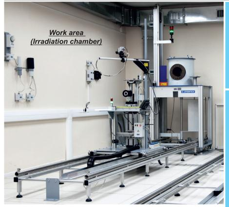
Reference AT140 Neutron calibration facility is designed to simulate and transmit neutron flux density, ambient and individual dose equivalent rates of neutron radiation during calibration, verification and testing of neutron radiation monitors and dosimeters.
