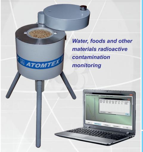
Highly sensitive selective wide-range spectrometric scintillation gamma activity monitor is intended for measuring volumetric (specific) radionuclide activity in <sup>131</sup>I, <sup>134</sup>Cs, <sup>137</sup>Cs, <sup>40</sup>K, <sup>226</sup>Ra, <sup>232</sup>Th samples with 1 litre Marinelli beaker and 0.5 litre and 1 litre flat containers.
