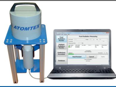
AT1135 Portable Radiometric Laboratory is a hand-carried measurement instrument of spectrometric type and is designed to determine relative activity of <sup>134</sup>Cs, <sup>137</sup>Cs and <sup>40</sup>K gamma-emitting radionuclides in food products as well as in-situ measurement of ambient gamma radiation dose rate equivalent.
